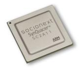
24x A53 1GHz cores @ 5W LPDDR4, PCIe G2 microATX 96Boards EE Upstream software support
